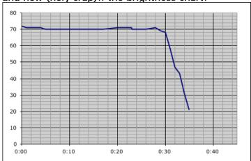
as you can clearly see.. HOLY COW! when used constantly, eventually the current sta dropping and the light cools off, which makes a marked improvement on the lumen/watt.. and basically exactly counteracted the dropping current up to 30 minute (the light was set to just about 400mA).. i will do a run test on a 'hotter' model soon.
