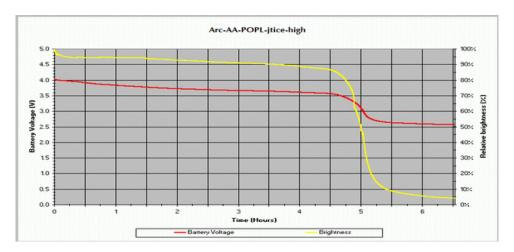
1Q: I noticed the initial drop of the brightness within a few minutes before settling at constant brightness in many run time tests. Is it something to do with the transistor/FET temperature change?
