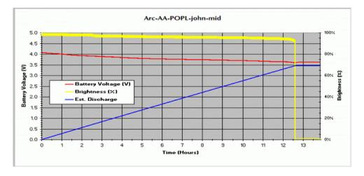
At first, I couldn't understand the sharp drop and sudden shutdown of the light after 12.5 hours. But the total estimated discharge at that time is 690mAh and imagine this no more juice left in the battery.
