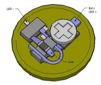
this is the identical circuit to the one above, done without any circuit traces... 'dead bug' style..
