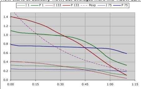
The green represents the '1W' version and the red represents the '1.5W' version. in addition there is a purple dashed line that represents a 1.6W straight-resistor model. The thin lines on the bottom are current.
