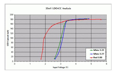
With the above componnts, it has to be called 45mV LDO-CC in my case. It is clear the constant current regulation is effective till Vin=3.4V with white led (Vf=3.2-3.3V) So at this current of 180mA, it should remain under regulation throughout the li-ion charge capacity (or at least 95%).
