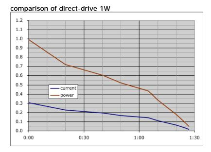
as you can see.. the DD model drops in 10min to the level the CC model holds for 45. pretty big difference.. notice that both models take about exactly 1 hr to reach 50% power.
